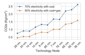
Figure 7: Carbon emissions for manufacturing cm<sup>2</sup> of silicon die for different technology nodes for two type of electricity generation schemes.
