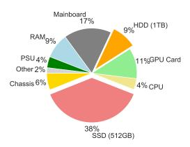
Figure 3: Distribution of embodied CO2e across different components of a Desktop system, data derived from [29].
