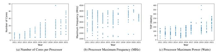
Figure 1: Intel Xeon processor trends across 447 CPU models. Each point represents an available Xeon CPU introduced in the given year. Despite the wide variation of configurations, core count is generally increasing per year while CPU frequencies and power demands have largely remained stable.
